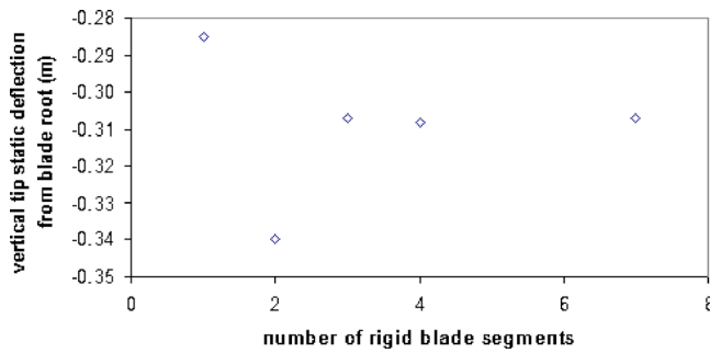
Fig. 8 Blade static deflection for experimental natural frequency with blade segmentation
